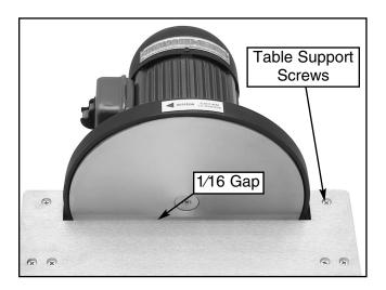
**Figure 7.** Table aligned with sanding disc.
